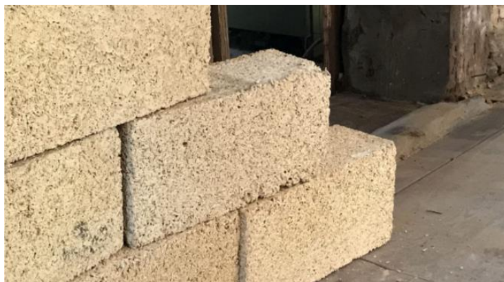
Figure 6: Hempcrete blocks for residential construction (Source: HempBuild Magazine)
