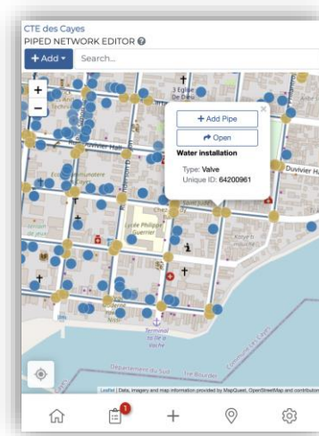
Figure 4. The mWater mobile app allows utility workers to view piped network infrastructure and add updates or new connections.
